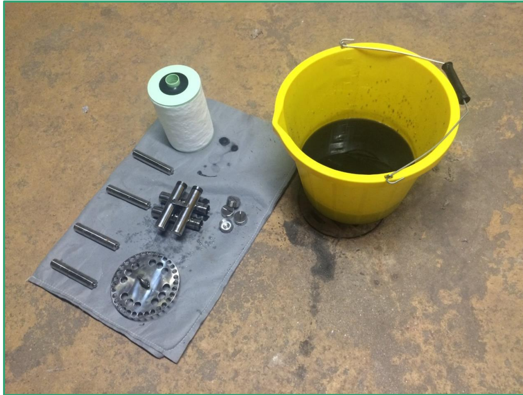
X-POT Magnet Grate post cleaning & new filter ready (15 minute process)
