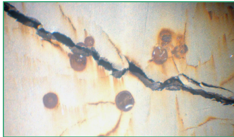
Stress corrosion cracking initiating from pit in austenitic stainless steel
