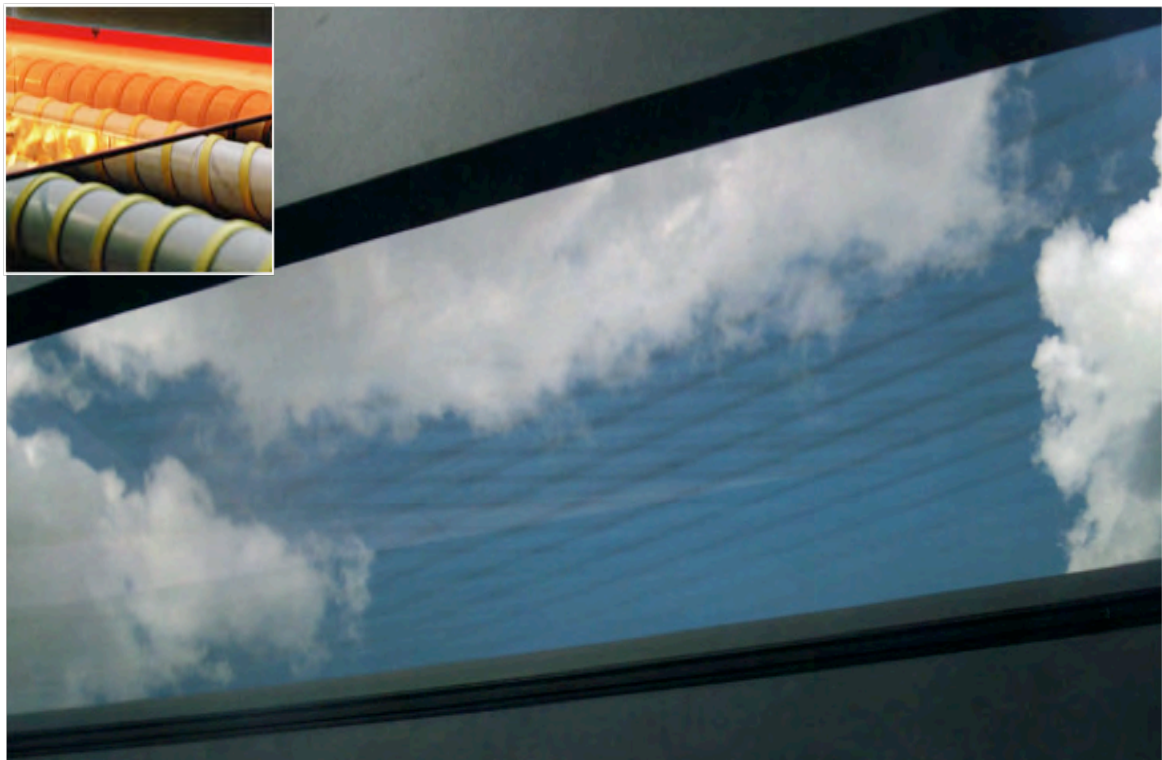
Figure 3.3.4: Anisotropy cross pattern (Henriksen and Leosson 2009) Inset: Spirally wounded support rollers (Glaston 2013)
