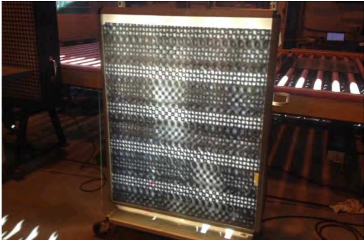
Figure 3.3.5: Anisotropy pattern on glass stationary during quenching (Vehmas 2014)
