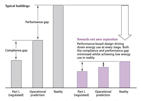
Figure 1.1 Energy performance modelling can help with dual aims: reducing the performance gap, and producing better, lower energy use buildings (image courtesy of Buro Happold)
