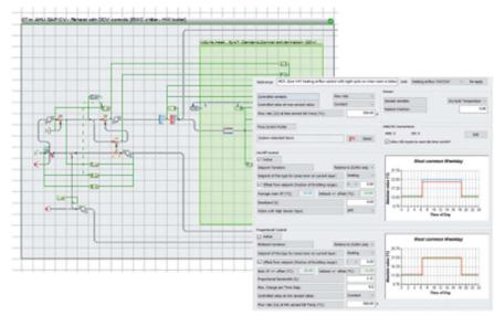
Figure 4.6 Illustration of 'template' and 'detailed' HVAC system modelling in IES software (courtesy of IES)
