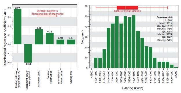
Figure 7.5 Example of parametric sensitivity and uncertainty analysis (courtesy of DesignBuilder Software)
