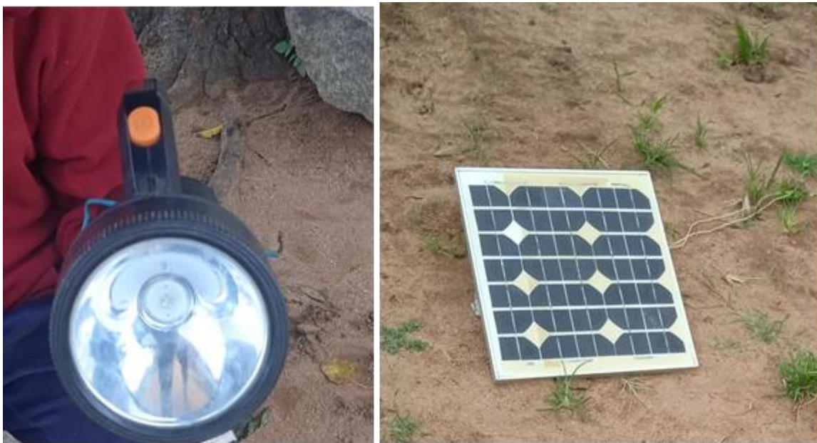
Figure 13: LED light with a separate solar panel
