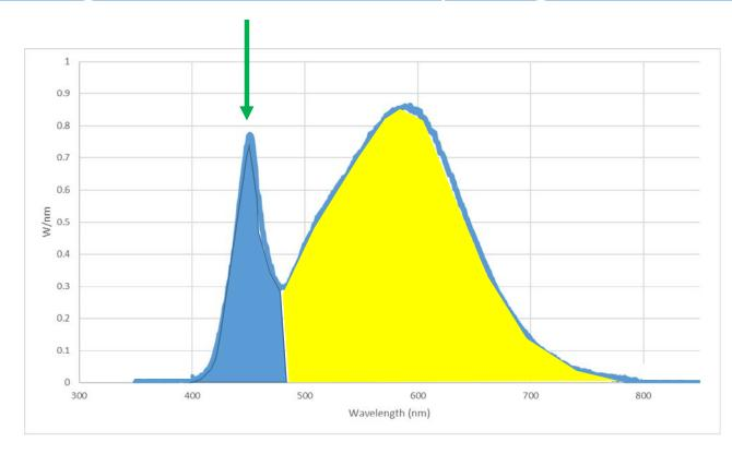
The blue LEDs used in street, office and domestic LED lighting generally emit at around 450 nm to 460 nm. For this reason, there are concerns that the guidelines may be exceeded......
