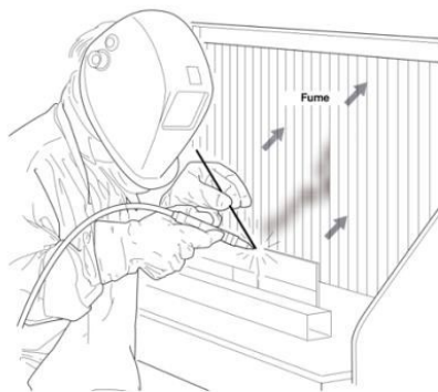
Welding table where the welding fume is captured and extracted by the airflow at the back
